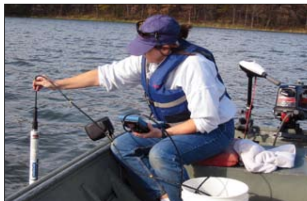
Multi-parameter meter measures dissolved oxygen, temperature, pH and conductivity.
